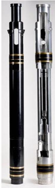
**Figura N° 4.** Bomba Jet Claw reversa
