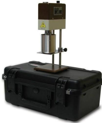
Fuente: OFI Testing Equipment – 130-10 Instructions – Viscometer, 8-Speed, Model 800
