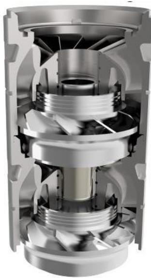
Figura 7. Bomba electrosumergible mixta
