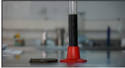
Figura 33. Filtrado OBM 30 mL 10 ppg, 120 lb/bbl de \text{CaCO}_3 malla 400/600.
