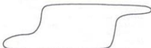
Combined Fluid Pound and Delayed Traveling valve closure
